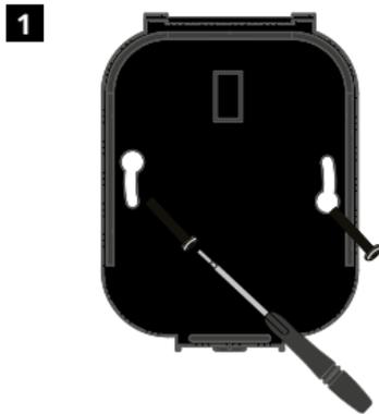
Insert fixing screws through mounting holes of the power base and tighten.
