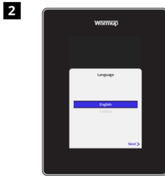
Re-attach the display until a “click” is heard. You can now restore power to the circuit and power up the thermostat. Follow the on screen instructions to set up your system. Once set up a QR Code will appear.
