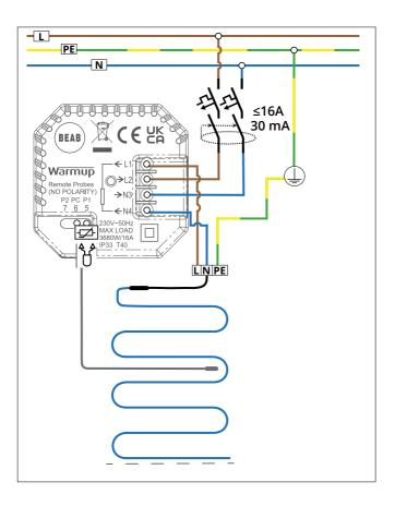
Warmup thermostats are rated for a maximum of 16 amps (3680 W at 230 V). A contactor must be used to switch loads exceeding 16 amps.
