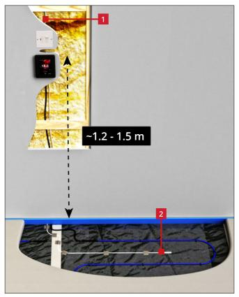
The supply to the thermostat MUST be protected by a 30mA RCD or RCBO at all times. Time delay RCD's or RCBO's must not be used. No more than 7.5 kW of heating should be connected to each 30 milliamp RCD or RCBO. For larger loads, use multiple RCD's or RCBO's.
